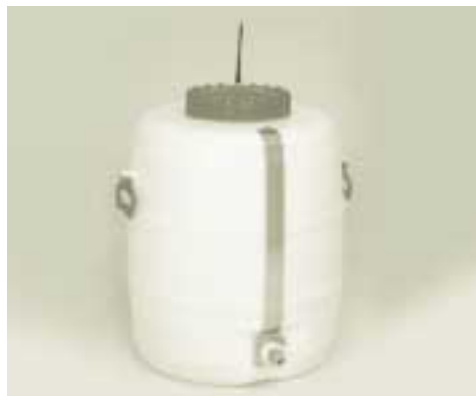
Spraying tank, UV light resistant polyethylene, 80 l, with mounting straps, level indicator, quick fit coupling for spraying hose, large filling and cleaning aperture, drain (only available for Mobilstar E and ER as optional accessory)
